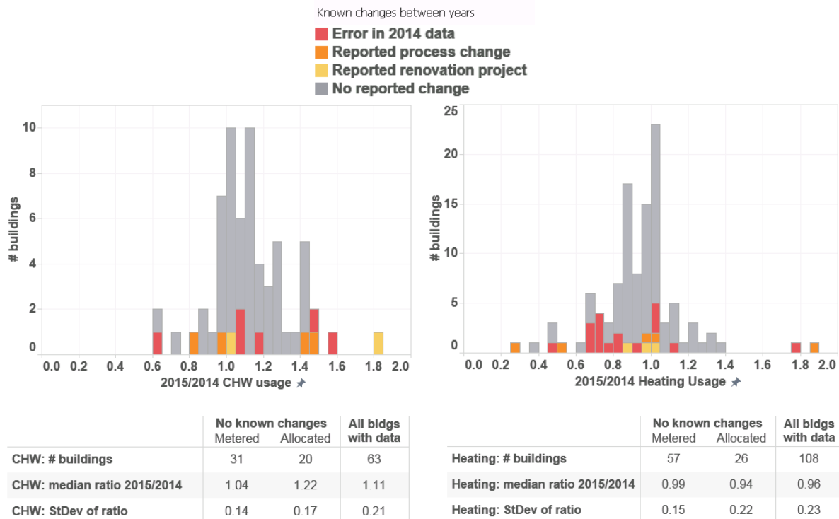
Figure 6: Distribution of ratios in chilled water usage (left) and heating source energy usage (right), with known changes highlighted
