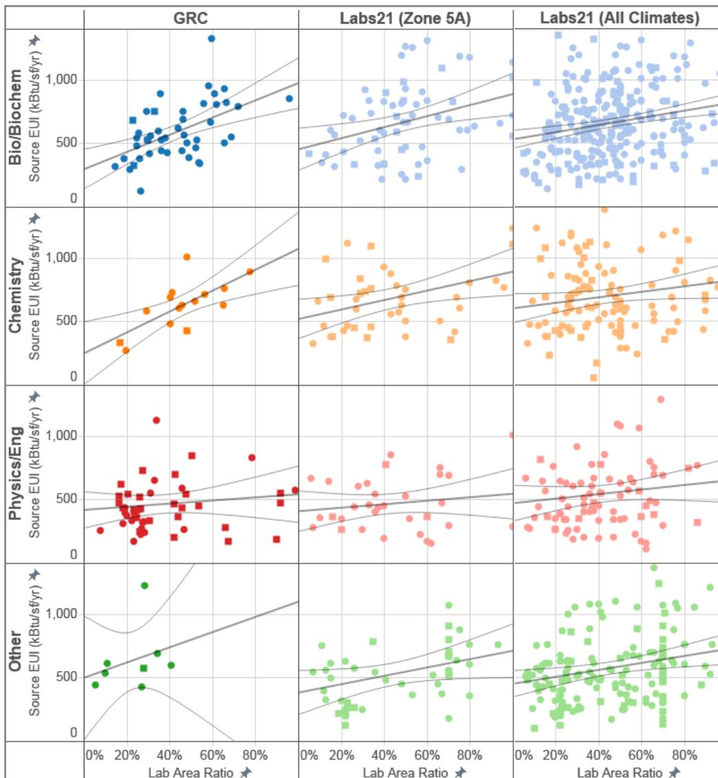
**Figure 12: Source EUI by Lab Type vs. Lab Area Fraction for the GRC sample (left), the Labs21 Climate Zone 5A Sample (middle), and the Full Labs21 National Sample (right)**
