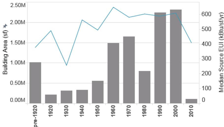
Figure 10: Building Area (Grey Columns) and Median Source EUI (Blue Line) by Decade Built for the GRC Sample (Fully Metered Data Only)
