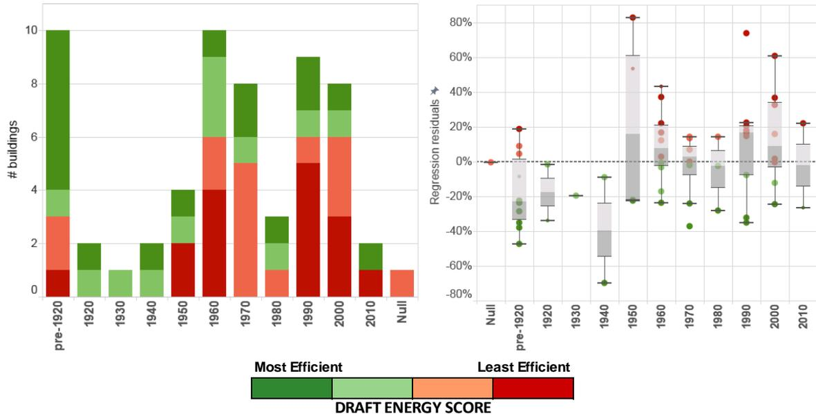
**Figure 15: Energy Ranking by Decade of Construction (Note: Left and Right Figures Show Same Data). Colors of Columns and Data Points Represent Energy Rankings.**
