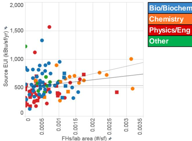
**Figure 13: Source EUI vs. Number of Fume Hoods Per Unit Lab Area for the GRC Sample**
