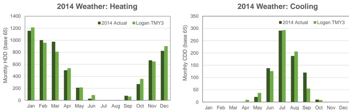
**Figure 3: Comparison of 2014 Boston Weather Data with Typical Meteorological Year (TMY3) Data**
